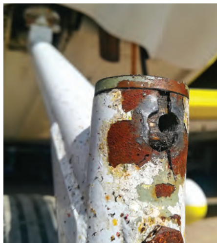
(Above) Here's a horror which was lurking unseen behind a SportCruiser's spat. LAA engine specialist, Kevin Hyam, came across this cracked spindle housing after removing the spat on a friend's machine. The aircraft is nine years old, had completed roughly 350hr and been fitted with the 'Dover spindle modification'. (Photo: Kevin Hyam)
