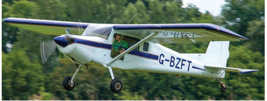
(Above) The Murphy Rebel is a two-seat, high-wing, all-metal monoplane which is available in kit form for amateur construction from Murphy Aviation Ltd, British Columbia, Canada. The Rebel is of conventional, riveted 6061-T6 sheet aluminium alloy, semi-monocoque construction and has a reputation for being a good short-field performer. A number of engine options are available – this example, one of the aircraft discussed in the main feature, is powered by the ubiquitous Lycoming O-320. The LAA has a total of 24 of these aircraft on our books, eight currently flying and ten of which are still under construction. (Photo: Tom Cole)
