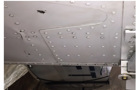
(Above & above right) The sketch above shows the numerous panels which go into a metal aircraft, and the one that’s showing cracking and needs either replacing or repairing can be seen in above right. It may be that the cracking along the rivet line is due to an overstress event at some time in the past, perhaps a heavy landing, possibly the recorded ground-loop, but both the repair and the replacement options will require the airframe to be completely stripped out and the fuselage held in a jig during the work. Fuselage structures lose their rigidity very quickly when panels are removed and it’s easy to damage unsupported structures, which is why a repair process needs much planning before any work begins.
