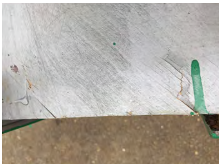
(Above) This is an example of fracture damage, most likely caused by the bursting effect of a compressive overstress, in the plywood skin of the Jodel's main spar. Because this aircraft has a section of false rib over the spar, to maintain wing top surface profile, this damage would be difficult to spot without close examination. (Photo: Alan James)
