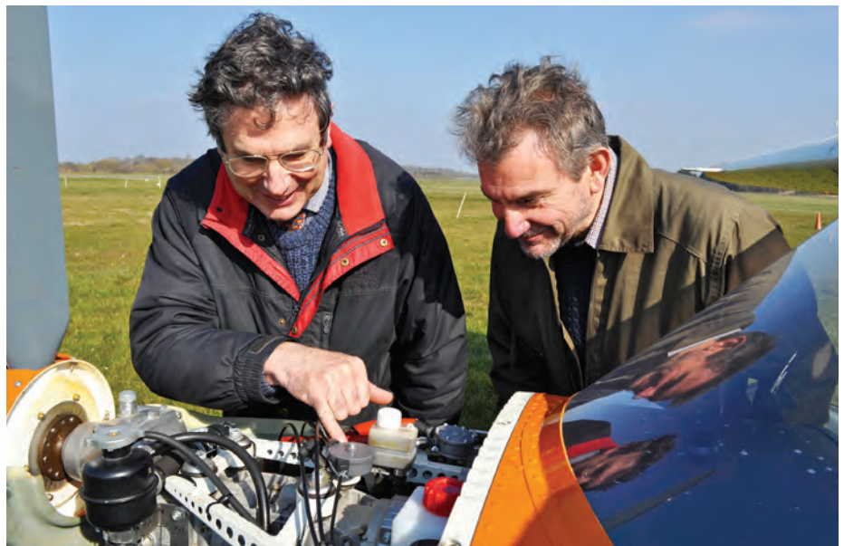
(Above) LAA Chief Engineer, Francis Donaldson, carrying out the duplicate inspection for LAA Inspector Graham Smith after an 'in the field' adjustment of an engine control. Whenever a flying or engine control is disturbed, for any reason, then it's essential that it's checked by a qualified second party before the aircraft is released for service. (Photo: LAA Engineering)
